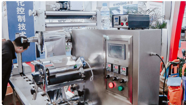
Blister packaging machine ready to be packed with capsules in flou-pack bags
