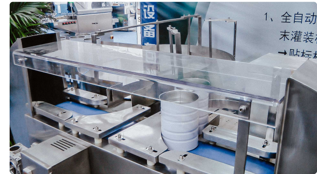
Food powder dosage and filling equipment in metal cans with capping metal lid
