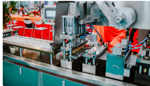
Automatic blistering machine for batch products honey, ketchup, jam
