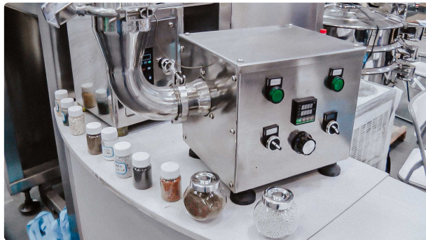
Laboratory machine granulator with powder and granule drying system
