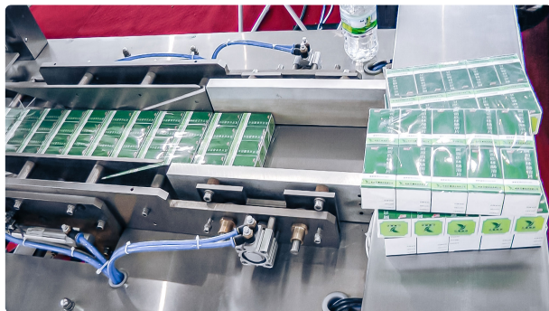
Automatic equipment cellophanator in pharmaceutical production
