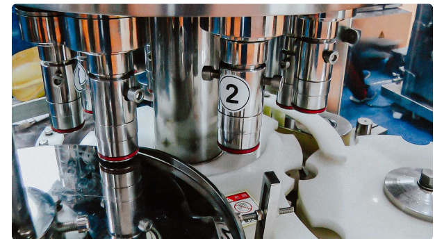
Automatic equipment for filling liquid products in a plastic syringe
