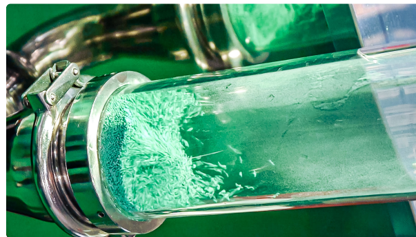
Automatic equipment for wet granulation of powders into granules
