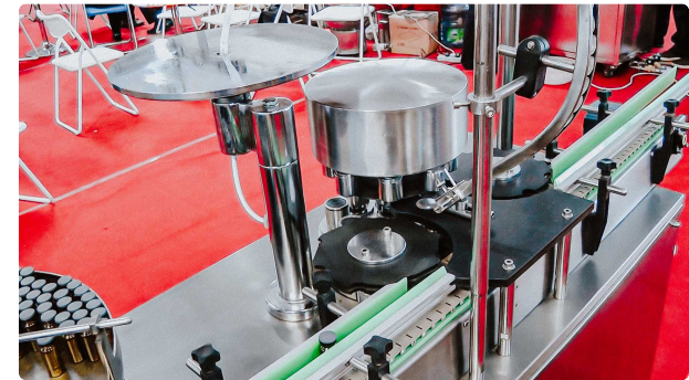
Automatic penicillin bottle capping machine with aluminum cap
