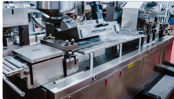
Pharmaceutical equipment for automatic packaging of tablets and capsules with...
