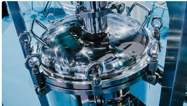
Homogenizer for gel and cream preparation in the cosmetic and pharmaceutical industry
