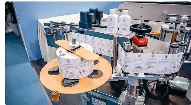
Automatic labeling equipment for sticking labels on both sides of flat bottles
