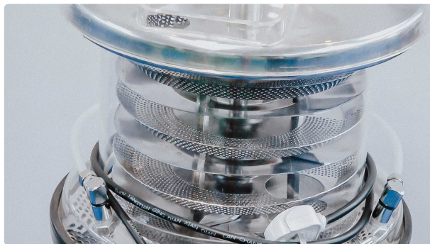
Vibration machine for dust removal from tablets and polishing after tablet production
