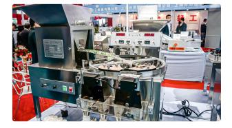
Automatic equipment for counting and packing of gelatin capsules into bottles Spain
