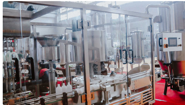
Automatic bottling machine for large plastic bottles and screw cap closure
