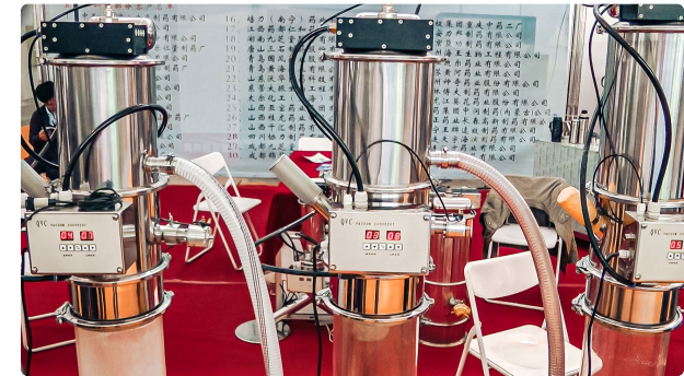
Automatic equipment for vacuum transport of powder in pharmaceutical production Portugal Pharmaceutical Tablet Press · 09.12.2020 · 174.500K views
