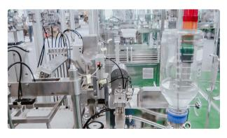
Automatic machine assembly and capping plastic syringes
