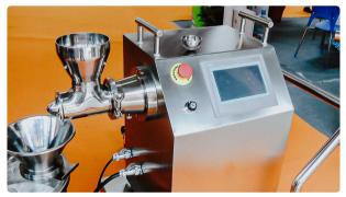
Automatic granulator with the function of pelletizing pellets to a round shape
