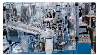
Automatic dispenser for cream and liquid filling of plastic tubes seal and release date
