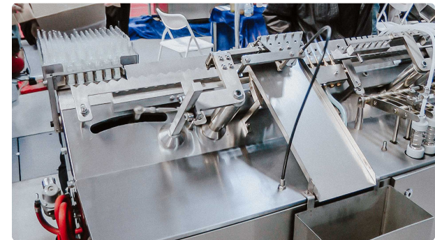
Automatic equipment for filling with liquid and sealing sterile glass ampoules with medicine
