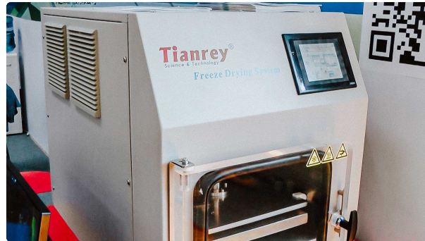
Sublimation lyophilic dryer for powder production from food and pharmaceutical...
