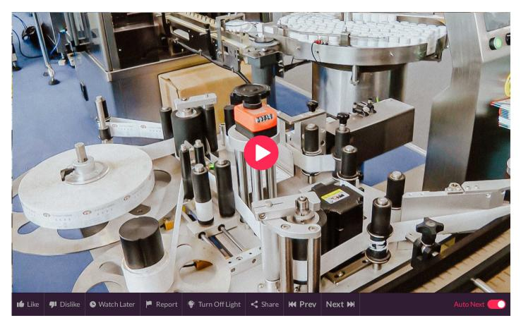
High speed automatic packing line for packing gelatine capsule into plastic bottles label sticker
