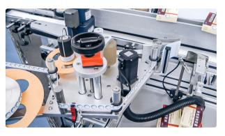
Automatic equipment for sticking self-adhesive labels on cardboard boxes of pharmaceutical...
