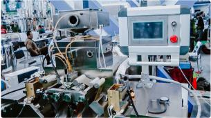
Pharmaceutical equipment for the production of soft gel gelatin capsules with oil inside
