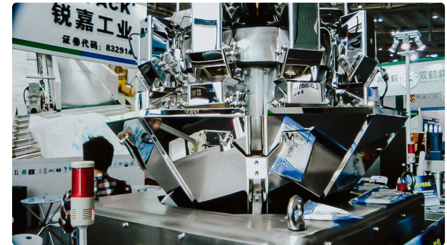
Multiple weigher for food and pharmaceutical packaging production
