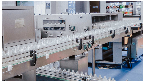
Automatic glass bottle washing machine and rinse aid in medicine filling line
