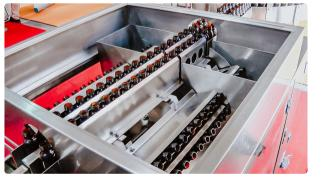
Automatic machine for washing and rinsing glass bottles with water for pharmaceutical... Pharmaceutical Packaging • 24.09.2020 • 100.050K views
