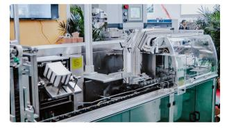
Automatic cartoning machine for packing blisters and plastic tubes into boxes
