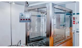
Automatic glass bottle washing machine in the filling and capping line
