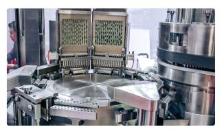
Automatic equipment for filling hard gelatine capsules with powder USA
