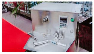
Automatic polishing moulds and punch machine for automatic rotary tablet press
