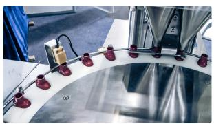
Automatic equipment for vibration feeding plastic bottles in pharmaceutical production
