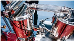
Automatic equipment for collection of pharmaceutical dust and powder residue
