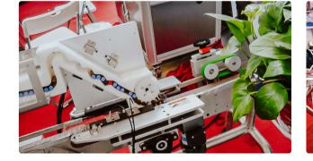
Automatic labeling equipment for labelling selfadhesive labels on glass ampoules and vials Pharmaceutical Packaging • 14.09.2020 • 698 views
