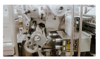
High speed automatic blistering machine for PVC / ALU packaging
