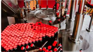
Automatic bottling and capping machine penicillin bottles with aluminum caps
