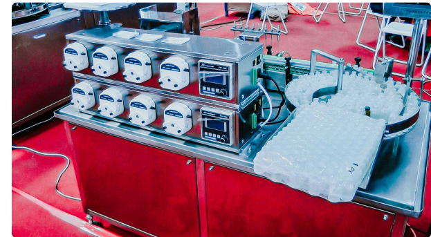
Automatic liquid filling machine for glass bottles with peristaltic pumps
