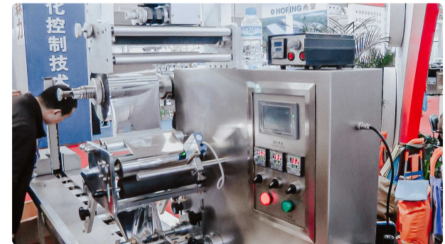
Blister packaging machine ready to be packed with capsules in flou-pack bags
