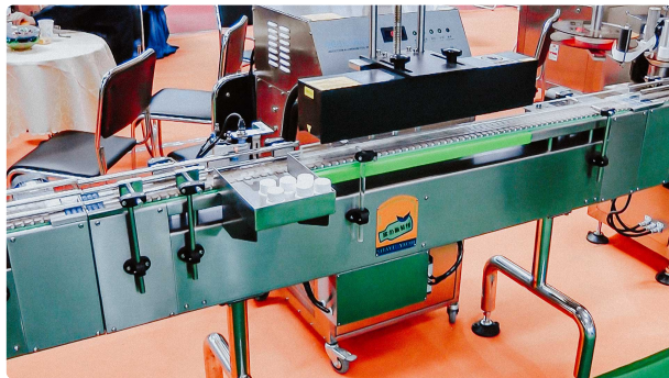
Automatic packaging line for tablets and capsules in plastic bottles capping and labeling
