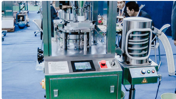
Laboratory tablet press for the production of pharmaceutical powder tablets
