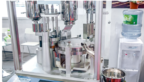
Automatic Powder Filling Equipment for Solid Gelatin Capsules
