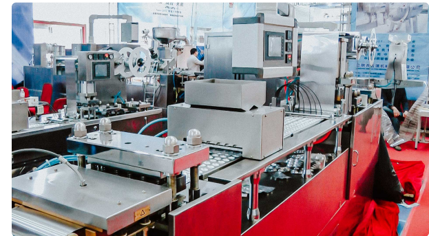
Automatic blistering machine for filling of tablets in blisters ALU / ALU
