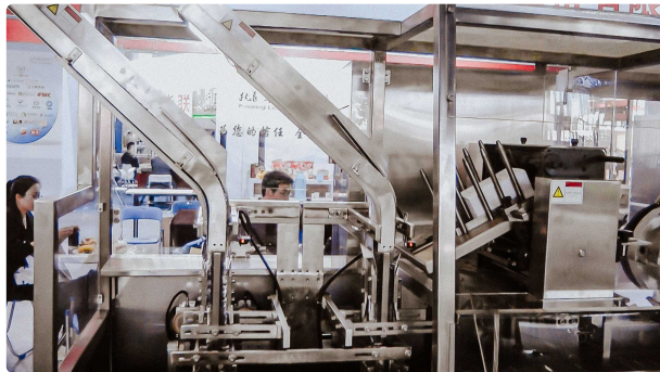
Automatic cardboard equipment for packing blister and products into boxes
