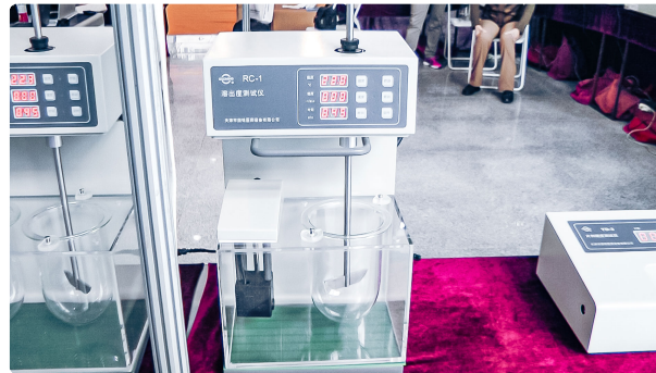
Automatic pellet speed testing equipment in pharmaceutical production
