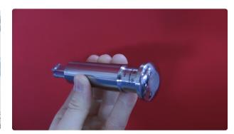
Punches and matrices for rotary tablet press samples
