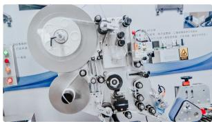
Automatic labeling machine for sticking labels on penicillin bottles
