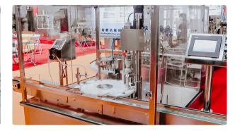
Mono block for filling and capping spray nozzle for plastic bottles
