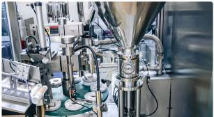
Automatic equipment for filling and sealing of cream in plastic tubes of pharmaceutical...
