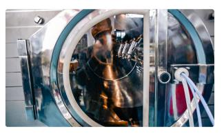
Automatic coating equipment for tablet surface application
