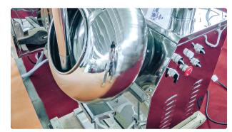
Automatic casing spraying equipment for tablet surface in pharmaceutical production
