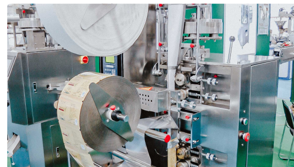
Automatic high speed packing machine for packing tea in filter bag and plastic envelope
