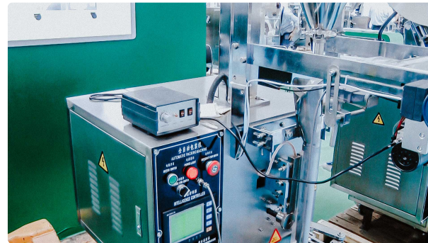
Automatic powder filling machine in plastic bags sticks
