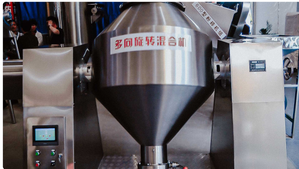
Automatic rotation cone for mixing powders in pharmaceutical factory
