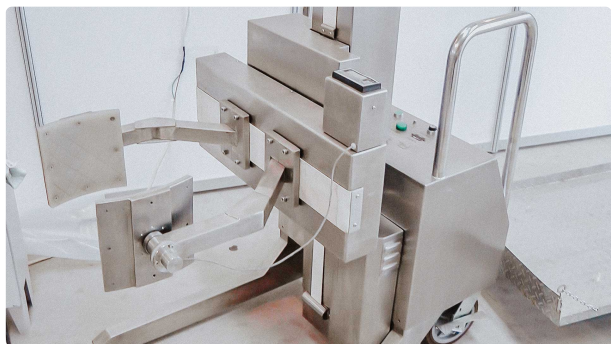
Automatic pharmaceutical pick-up for powder containers
