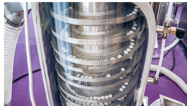
Automatic equipment for cleaning and polishing of tablets in pharmaceutical production
