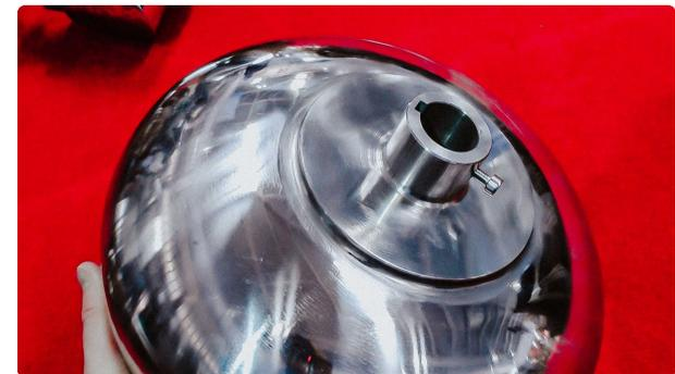
Coater for applying the tablet shell for pharmaceutical laboratory drug manufacturing
