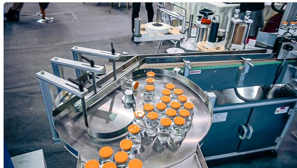
Automatic equipment for sticking self-adhesive labels on the glass bottles
