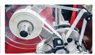
Automatic labeling equipment on top of cardboard boxes in pharmaceutical production
