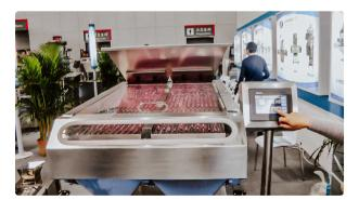
Automatic tablet filling and counting machine in plastic bottles
