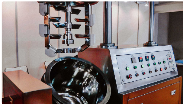
Pharmaceutical homogenizer for cream and emulsion preparation in cosmetic production
