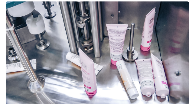
Automatic equipment for filling of cream and ointment in aluminum tubes in pharmaceutica...
