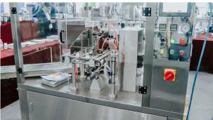
Automatic capping machine for high unstable bottles and screw caps
