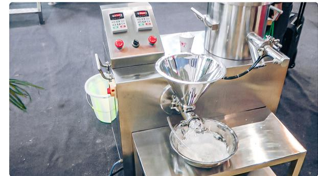
Automatic equipment for obtaining granules from powders by pharmaceutical production
