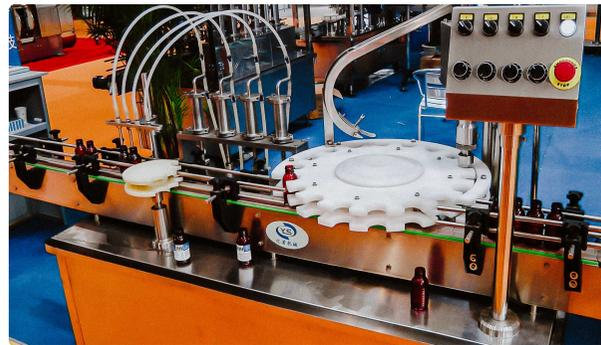
Automatic equipment for filling liquid products in plastic bottles with capping caps
