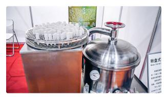
Automatic equipment for obtaining granules from wet powders
