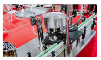
Automatic penicillin bottle capping machine with aluminum cap
