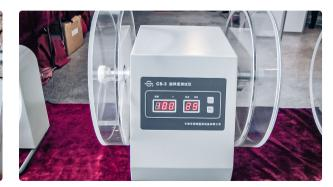
Automatic equipment for testing the abrasion rate of tablets and capsules in pharmaceutical...
