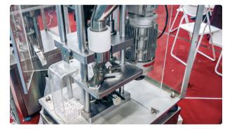
Automatic equipment to make tablets using tablet press in pharmaceutical production
