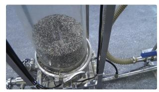
Powder vacuum conveyors for working with various pharmaceutical equipment
