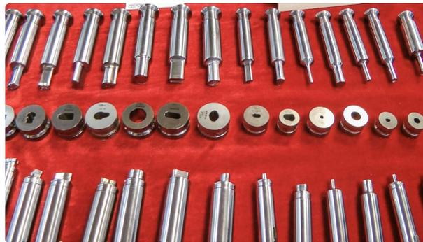
Mould for rotary tablet press tablet pressing from pharma powder
