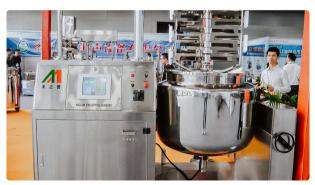
Homogenizer tank with blade system mixing liquid and powder for cream
